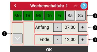
The weekly timer has the following setting options, day of the week (①), start time (②) and end time (③). 3 time windows can be defined per timer. You can switch between them with the arrow keys (④).
