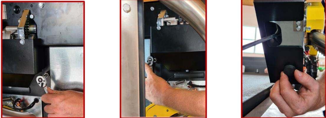
Figure 11: Removal of the front cover
