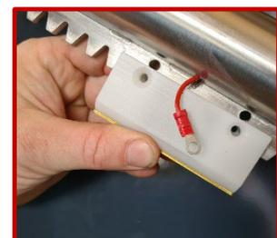
Figure 16: Connection of positive cable on the charging point
