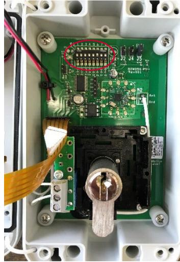
Figure 19: Outdoor control circuit board
